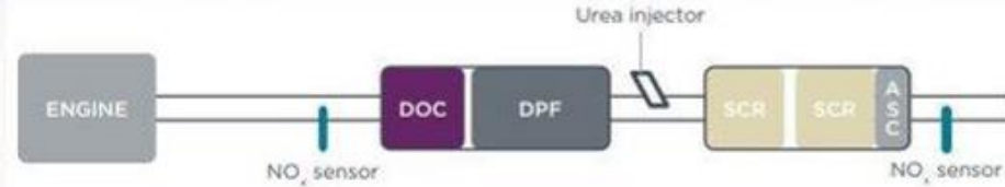
Figure 1. EPA 2010 aftertreatment system layout.
